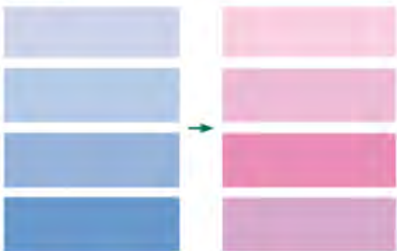
Distinct change of color: New Class 1 process indicator according to ISO 1140-1:2014. It displays a clear change of color from blue to pink.
